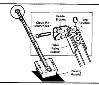
PROCEDURE: Position opener chassis on garage floor below the header bracket. Use packing material base to protect cover. NOTE: To enable the Tee rail to clear sectional door springs, it may be necessary to lift the chassis onto a temporary support.
